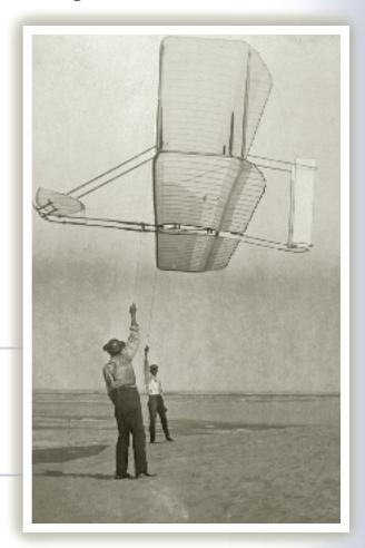
Orville and Wilbur controlled their first airplane by pulling on strings connected to the wings.
